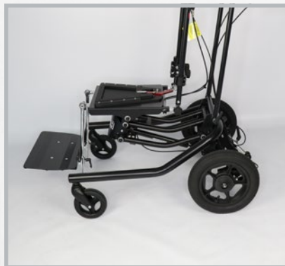
Height adjustment to lower the seat down to the ground
