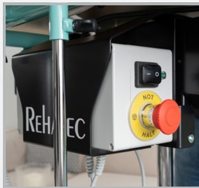
New electric drive with emergency stop button
