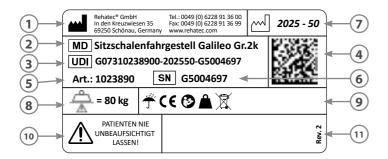
The illustration shows an example type plate. The serial number shown does not correspond to that of your device.
